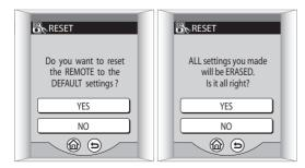
After the screen goes blank, the Home menu appears within a minute or so, and the remote control will be reset to the default settings.
